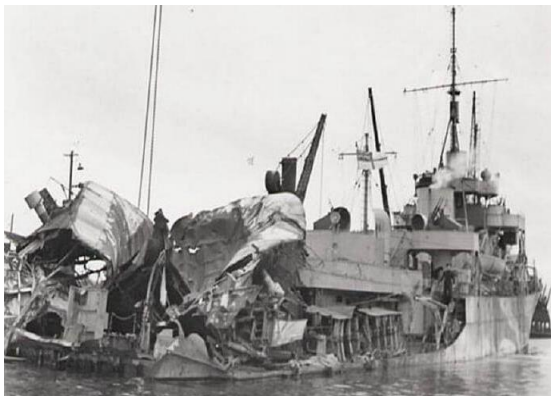
Torpedo Damage to HMCS Chebogue Source: https://valourcanada.ca/
