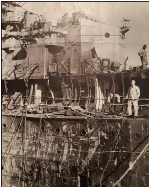
Damage to HMCS ATHABASKAN G07 caused by a glider bomb attack on August 27, 1943. Source: From the collection of Joseph W. (Jim) L'Esperance, LS, RCNVR, For Posterity's Sake website.
