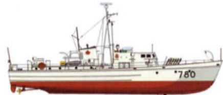
Bird Class HMCS Loon 66 tons - 28 m x 5.2 m x 1.6 m - 14 kt
