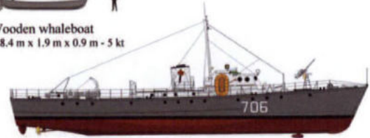
Fairmile-B Class HMCS Beaver (II) 79 tons - 34.1 m x 5.4 m x 1.5 m - 20 kt
