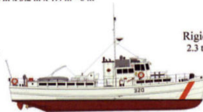
75-foot YAG Class YFB-320 81 tons - 22.9 m x 5.6 m x 1.2 m - 11 kt
