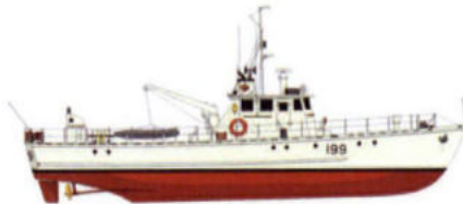
75-foot Detachment Class Standoff PB-199 70 tons - 22.9 m x 5.2 m x 1.8 m - 15 kt
