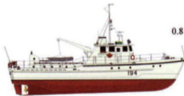
65-foot Detachment Class Acadian PB-194 45.5 tons - 19.8 m x 4.5 m x 1.7 m - 10 kt
