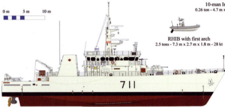
Kingston Class HMCS Summerside (II) MM-711 970 tons - 55.3 m x 11.3 m x 3.4 m - 15 kt
