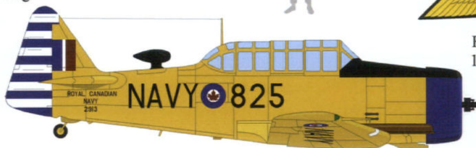
North American Harvard 290 km/h - 12.8 m x 8.8 m x 3.5 m Crew of 2 2913 / 825 VC 923 Squadron Québec City - 1956
