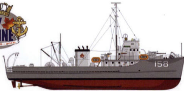
YMS-400 Class HMCS Cordova 325 tons - 41.5 m x 7.5 m x 2.4 m - 15 kt
