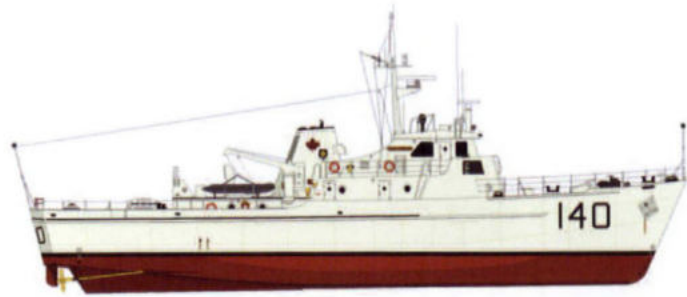
HMCS Fort Steele PB-140 85 tons - 36 m x 6.4 m x 2.1 m - 20 kt
