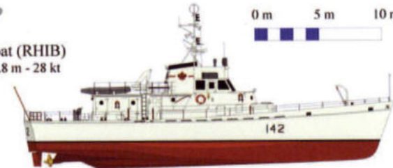
"R" Class Rapid PB-142 119 tons - 29.1 m x 6.1 m x 2.2 m - 20 kt
