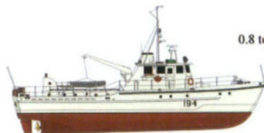
Classe Detachment de 65 pieds Acadian PB-194 45.5 tonnes - 19.8 m x 4.5 m x 1.7 m - 10 nd
