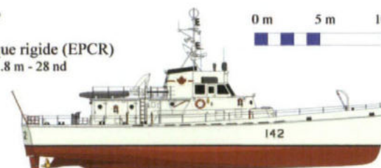
Classe "R" Rapid PB-142 119 tonnes - 29.1 m x 6.1 m x 2.2 m - 20 nd
