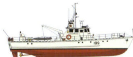
Classe Detachment de 75 pieds Standoff PB-199 70 tonnes - 22.9 m x 5.2 m x 1.8 m - 15 nd
