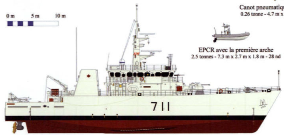
Classe Kingston NCSM Summerside (II) MM-711 970 tonnes - 55.3 m x 11.3 m x 3.4 m - 15 nd
