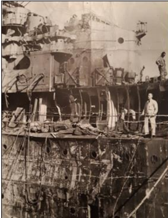
Battle Damage Damage to HMCS Athabaskan caused by glider bomb 27 Aug 1943.
