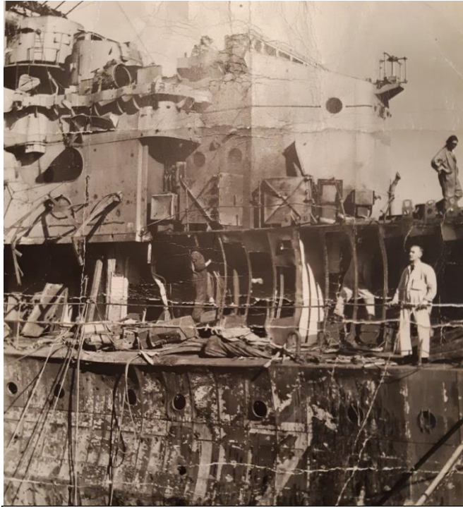
Damage to HMCS Athabaskan caused by glider bomb 27 Aug 1943. Photo credit: From the collection of Joseph W. (Jim) L'Esperance, LS, RCNVR ( www.forposteritysake.ca )
